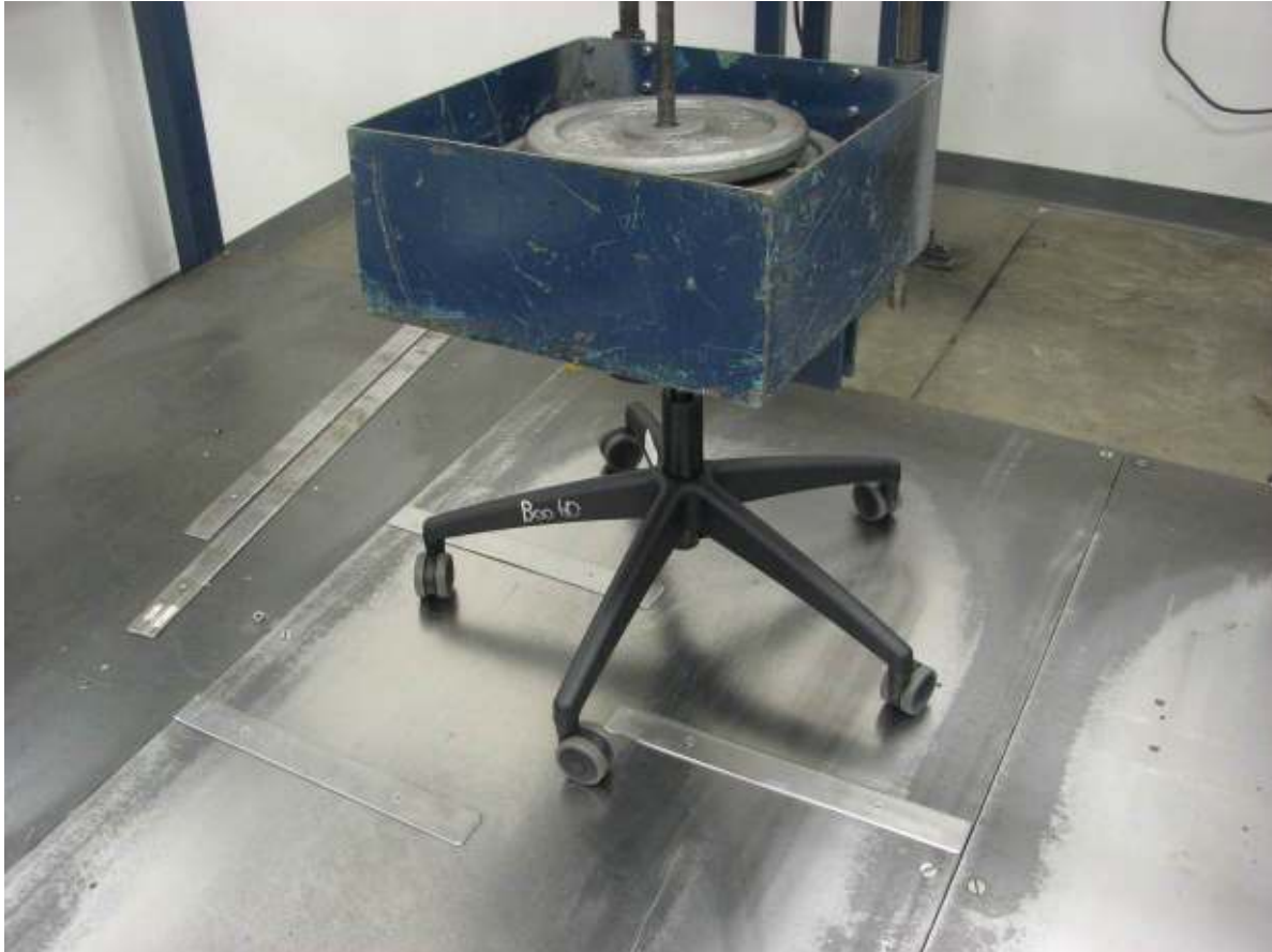
Caster/Chair Base Durability Test - Cyclic
