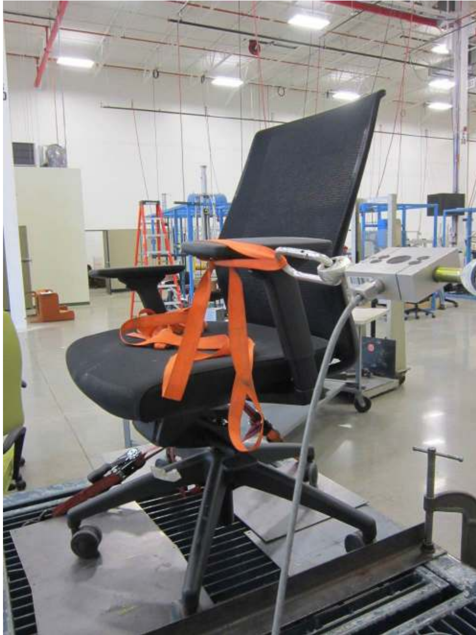
Arm Strength Test- Horizontal-Static
