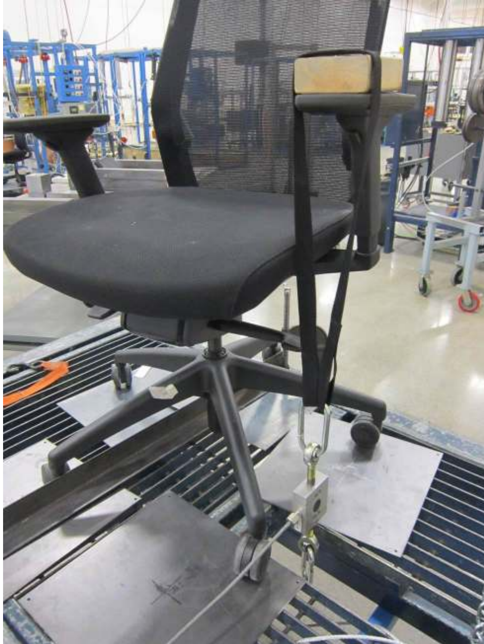
Arm Strength Test Vertical-Static
